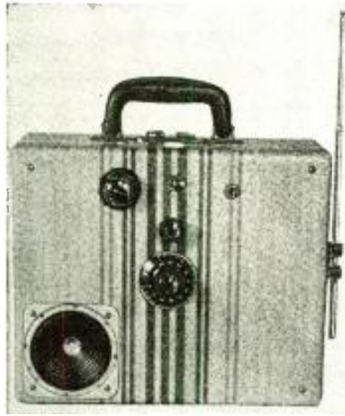
A dandy portable battery receiver—it uses one tube and gives loud-speaker reception.
